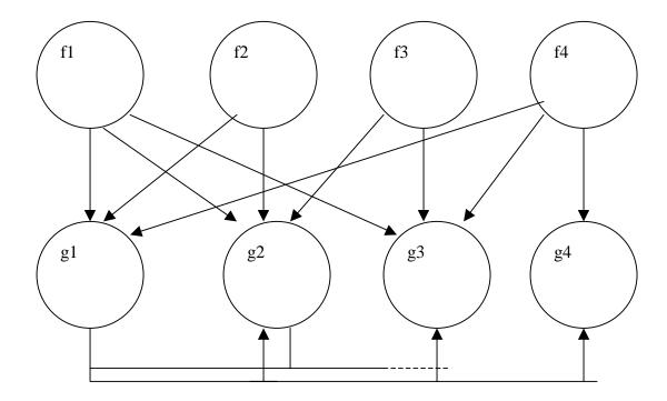
A network computing the full set of 4 PCs g1, g2 etc from the 4 input neurons f1, f2 etc. The left postsynaptic cell computes the first PC etc. Not all the feedforward and lateral (recurrent) connections are shown
