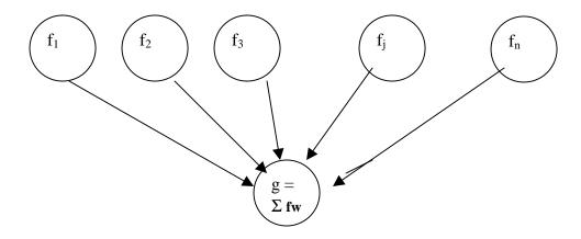
Idealised connectionist neuron. The neuron gives an output g which is the sum of its weighted inputs  $f_i$ .
